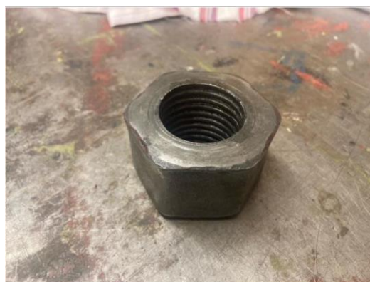
Brake adjuster nut with worn thread
